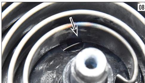
All the parts in movement, including the springs, must be well lubricated. Now go on by charging the return spring: take the head of the rope leaving 10-20 cm coming out the hole with "u" shape on the wheel side. Turn the wheel three times in counter clock-wise sense till it stops in front of the exit hole on the aluminium case. Keeping the plastic wheel stopped, pass the rope through the case hole. Insert the handle and the washer and tie a single knot as shown in photo 9.
