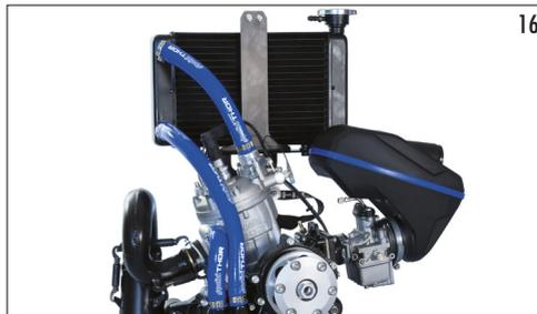
Fix the big bracket supplied between the two vibration-dumping mountings at the top and the frame. Fit the two rubbers on the bracket and place the radiator. To fix the radiator in the top side a bracket and a rubber are provided.
