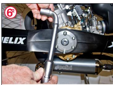
We use a tubular bent key of 19mm. which is the only key that will let you fasten with strength without damaging the central bolt.
