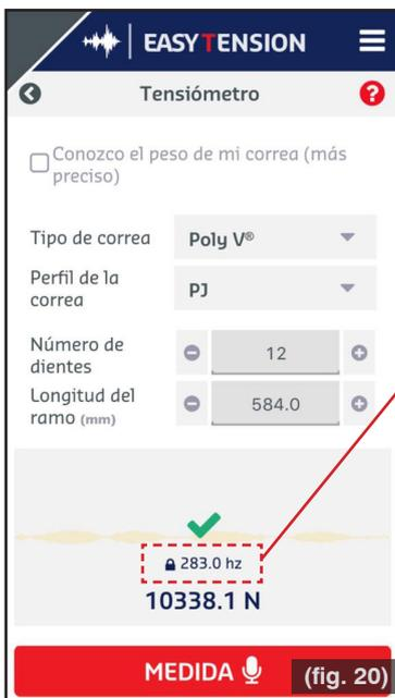
**COURROIE AVEC PEU DE TENSION. IL EST OBLIGATOIRE DE LA TENDRE.**
