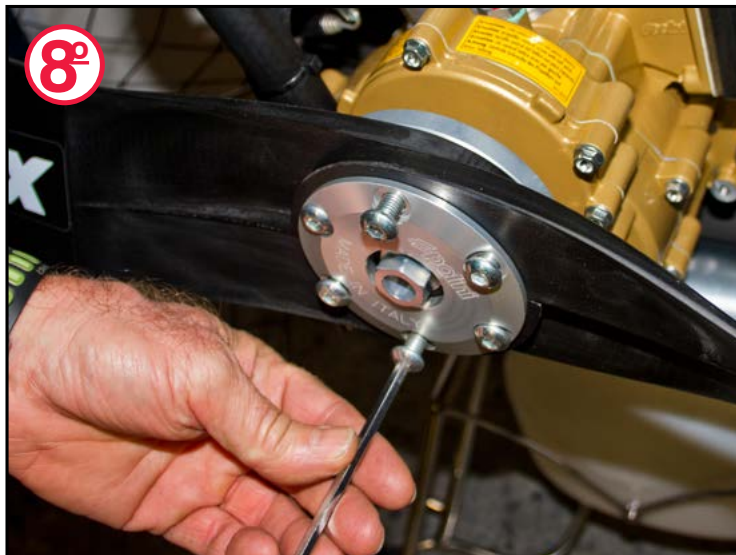
Fasten the 6 screws of the carbon propeller at 0.8 Kgm (8Nm).
