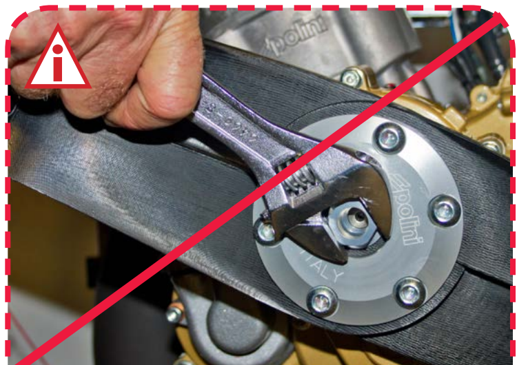
DO NOT USE ANY OTHER KEY TO FASTEN FOR NOT DAMAGING THE CENTRAL BOLT AND BE ABLE TO TIGHTEN WITH STRENGTH.
