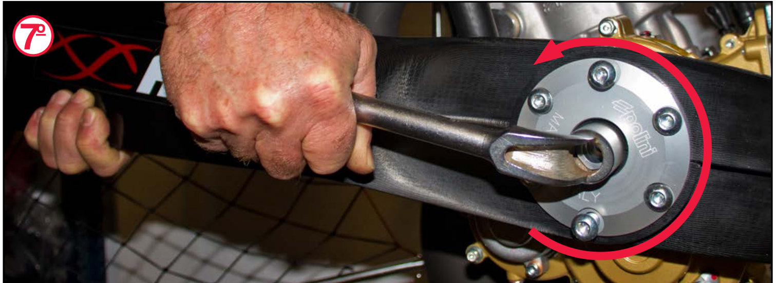
Fasten *anti clockwise while we hold the propeller with our other hand.
