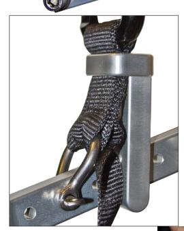
Remember that now the balancing point is the top part of the ATS where the paragliders attachment loop goes through , so moving the shackle has no influence in your position during flight.
