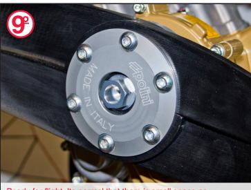
Ready for flight. Its normal that there is small space no bigger than a millimeter.
