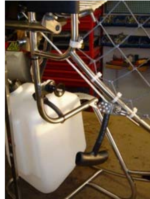
Positioning the pull start cord in the 4 or 5 part chasis
