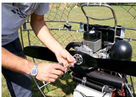
::: N. 27 ::: ::: HELICE: CONTROL Y APRIETE ::: ::: PROPELLER: RE-TIGHT AND CONTROL :::
