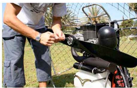
::: N. 27B ::: ::: HELICE: APRIETE Y REVISION ::: ::: PROPELLER: TIGHT AND RE-CHECK :::
