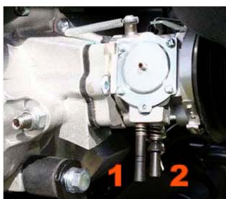
::: N. 25 ::: ::: CARB. WALBRO: AGUJAS DE REGULACION ::: ::: WALBRO CARB: SETTING CONTROLS :::
