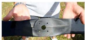
::: N. 21B ::: ::: HELICE FIBRA CARBONO ::: ::: CARBON-FIBER PROPELLER :::
