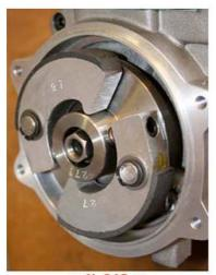
**::: N. 24C :::** ::: EMBRAGUE CENTRIFUGO ::: ::: CENTRIFUGAL CLUTCH :::
