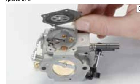
**ATTENTION:** The carburetor is made of many small and fragile parts. Be very careful during all the phases with particular attention to the idling and its springs; they both must not be touched.
